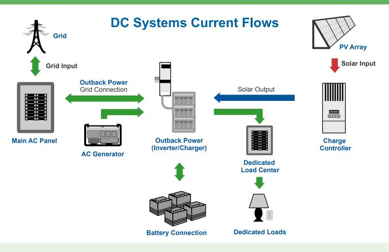
Our small systems are ideal for most residences with 3600 Watt, 120VAC output. These systems are prewired for fast and clean NEC compliant installation and the included solar charge controller can accept up to 4 kW of solar power.
