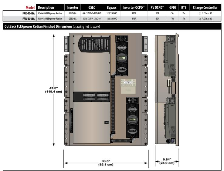
\*All pre-wired systems include a Radian Series inverter/charger, FLEXmax 80 charge controller(s), MATE3 system display and communications, FLEXnet DC system monitor, AC and DC wiring boxes, HUB 10.3 communications, surge protector and remote temperature sensor (RTS). The FLEXpower Radian is also equipped with battery and PV array breakers, GFDI and input-output-bypass. See individual product specsheets or product guide for full specifications. \*\*Overcurrent protective device.
